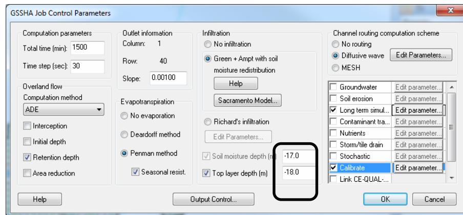
So, altogether there are 18 parameters that will be used in the automated calibration, we have 14 storm events and we will let GSSHA run a maximum of 500 simulations. The model is all set up to run an automated calibration.
