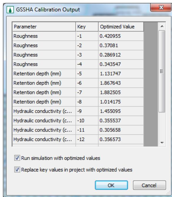
3. Click OK to replace the key values for calibration (all the negative numbers) with the optimized parameters and run GSSHA.
